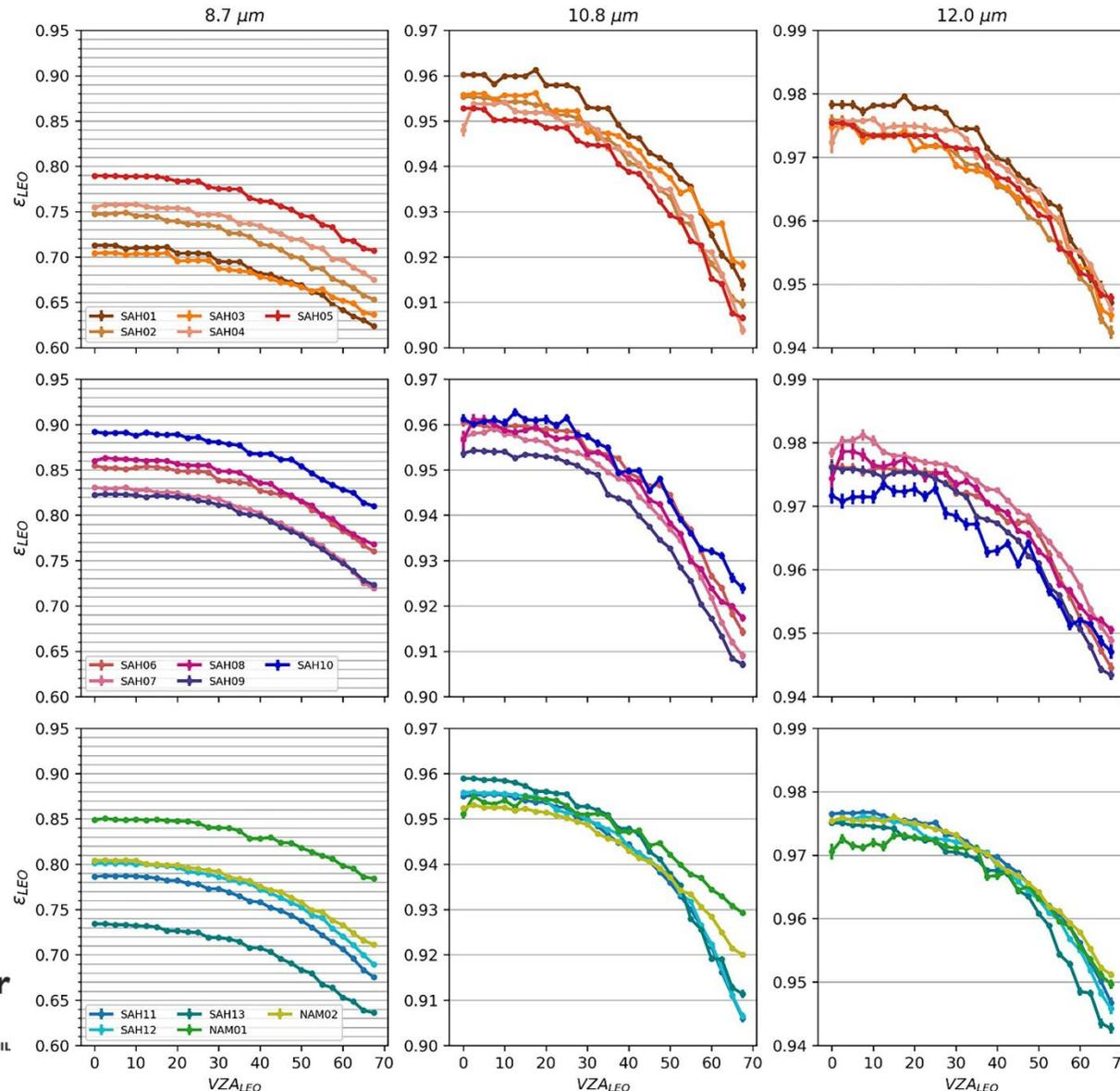
Fig. 4. Multi-sensor retrievals of angular dependence of LEO emissivity ( $\epsilon_{LEO}$ ) as function of LEO VZA (degrees) at the selected sites (represented by the colors). From left to right: emissivities for channels centered at 8.7 μm, 10.8 μm and 12.0 μm, respectively. The error bars indicate the 95% confidence intervals of the regressions. The y-axes have different ranges, but the grid lines correspond to the same intervals in all plots.
