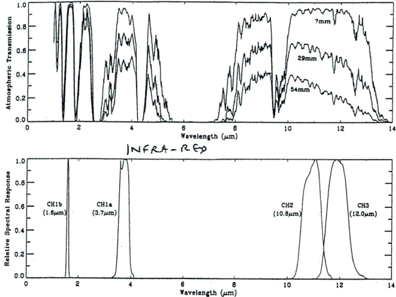
Figure 2.1: Atmospheric transmission for three different amounts of precipitable water (7mm — polar; 29mm — temperate; 54 mm — tropical), and the ATSR spectral channels matched to atmospheric 'window' regions.
