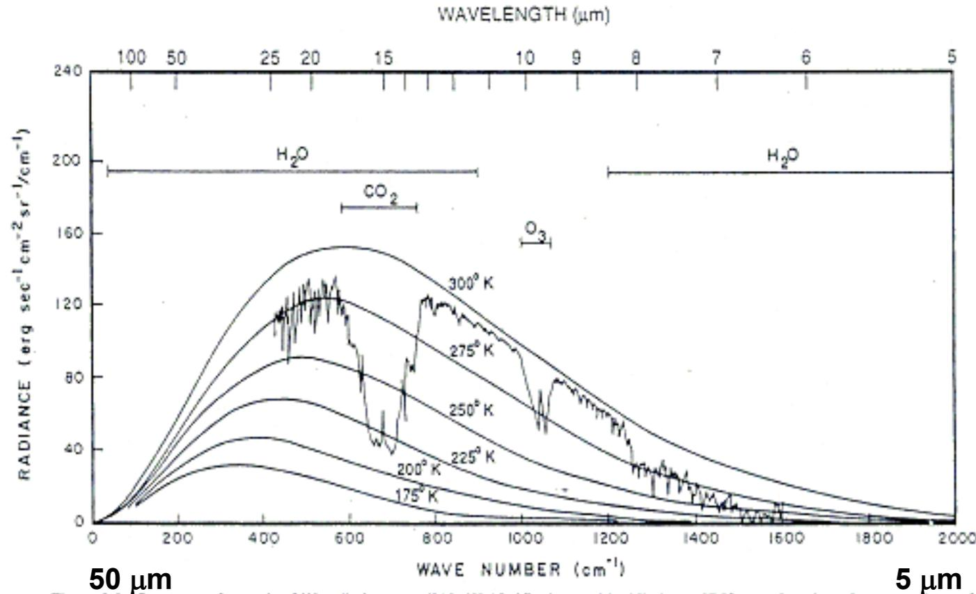
Figure 8.5 Spectrum of outgoing LW radiation over (215° W, 15° N) observed by Nimbus-4 IRIS, as a function of wavenumber  $\lambda^{-1}$ . Blackbody spectra for different temperatures and individual absorbing species indicated. Adapted from Liou (1980).
